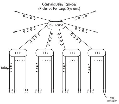
Figure 2-4. DNH-6800 DigiNet Hub Module (Large Network)
